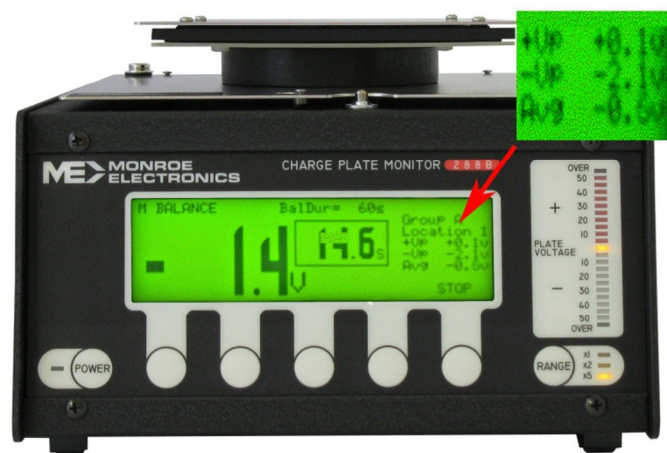
Figure 1. The Monroe 288B measuring ionizer balance.
