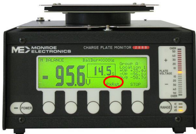
Figure 5. The CPM in the balance mode optimized for pulsed DC ionizer measurements.
