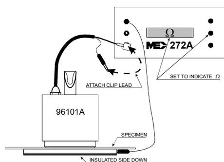
Figure 3: Setup for Guarded Measurement of Volume Resistivity
