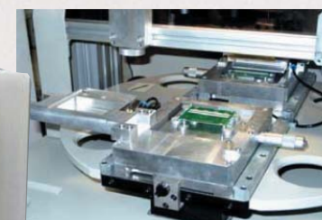
Rotary work feeder for fast load/unload. Operated manually or pneumatic power as option.
