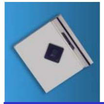
This tool allows the operator to visually inspect the coplanarity of a formed SMD. The operator looks down at the angled mirror to see two adjacent sides of the package at once. It has an optically perfect mirror, which is angled to make it easy to perform this inspection procedure. Small and compact, it measures only 4" x 4" and has a plated tool steel base. P/N CI-1.
