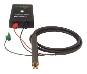
**Warning:** During use, excitation voltage appears between the two spring contacts. **DO NOT TOUCH THE CONTACTS!**
